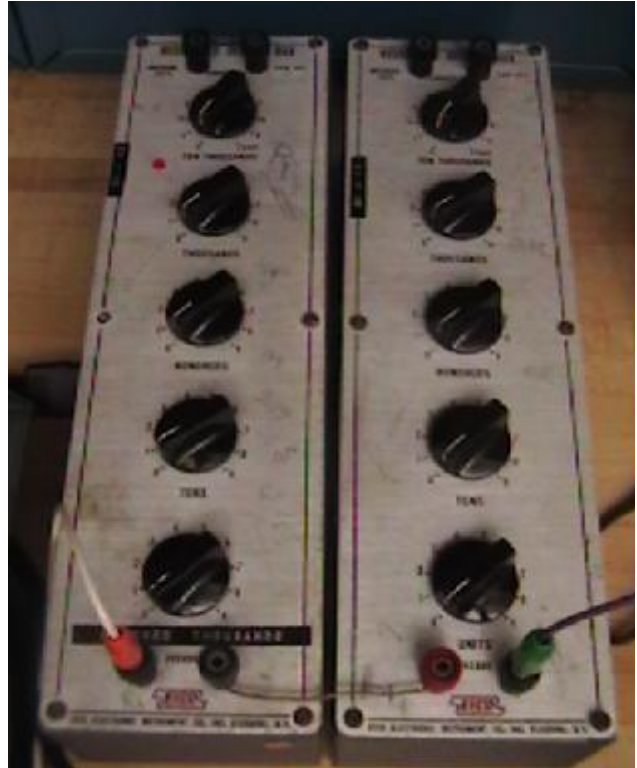
Figure 17: Two Resistance Decade Boxes Wired in Series.
